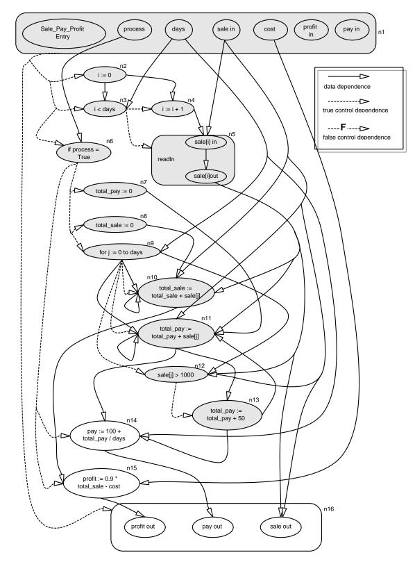
Figure 6: PDG for Sale\_Pay\_Profit program. The shaded nodes represent the slice on node n13.
