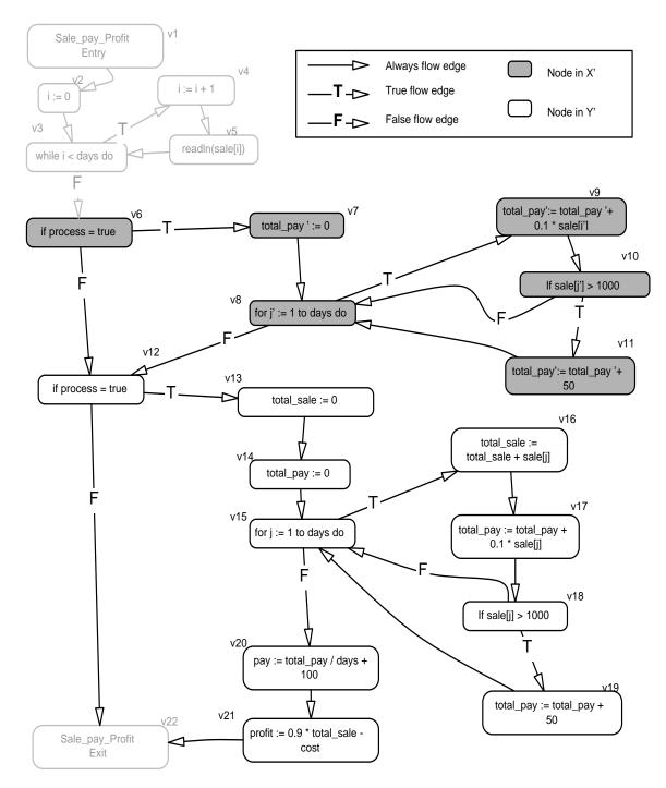
Figure 13: New CFG created by the first step of SPLIT. This is the solution for SPLIT using the result of TUCK from Figure 12.
