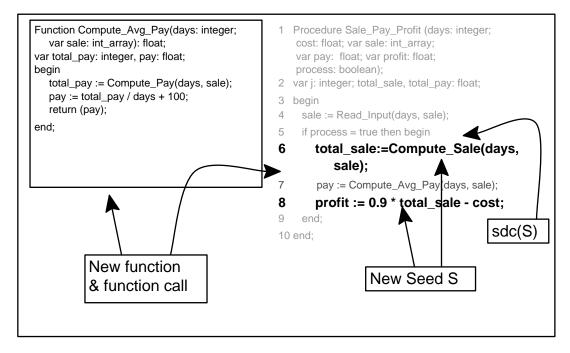
Figure 20: The average Pay is extracted from Sale\_Pay\_Profit. Now, lines 6 and 8 become the seed for the next restructuring. The sdc under consideration is on line 5 and the rc is defined by lines 6, 7, and 8.
