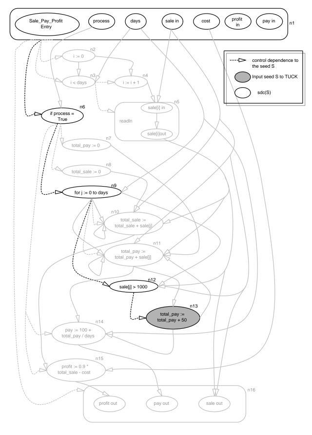
Figure 9: TUCK first computes the single definite control nodes (sdc) for the initial seed, n13. In this case, the seed is the singleton  $\{n13\}$  but generally it can be a set. The resulting set,  $sdc(\{n13\}) = \{n12, n9, n6, n1\}$ .
