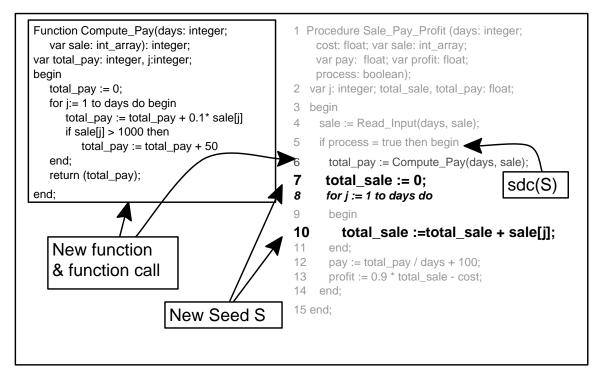
*Figure 18: Total\_Pay is extracted from Sale\_Pay\_Profit. Now, lines 7 and 10 become the seed for the next restructuring. The sdc under consideration is on line 5 and the rc is defined by lines 7,8, 9, and 10.*
