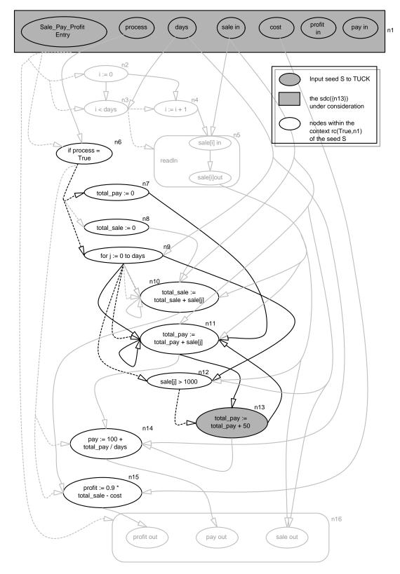
Figure 12:  $TUCK(\{n13\})$  within the restructuring context defined by n1. The slice on n13 within rc(True, n1) is  $\{n6, n7, n9, n11, n12, n13\}$
