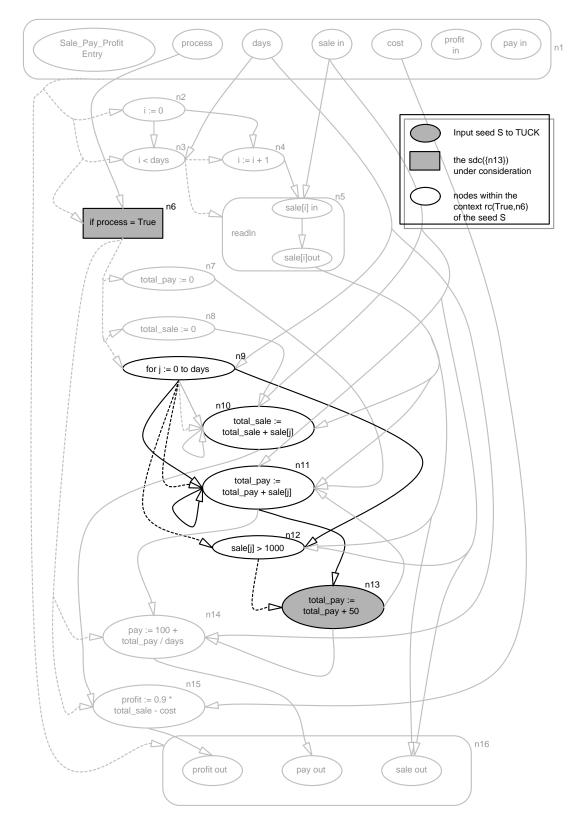
Figure 11:  $TUCK(\{n13\})$  within the restructuring context defined by n6. In this case the slice on n13 within rc(True, n6) is  $\{n9, n11, n12, n13\}$
