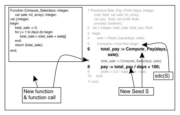
*Figure 19: Total\_Sale is extracted from Sale\_Pay\_Profit. Now, lines 6 and 8 become the seed for the next restructuring. The sdc under consideration is on Line 5 and the rc is defined by lines 6, 7, and 8.*
