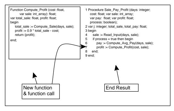
Figure 21: The end result is the function Sale\_Pay\_Profit semantically unchanged but now calling many smaller functions. Each of the function can become a method of an object in a object-oriented design.
