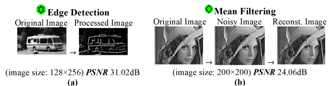
Fig. 5. Real applications of the cooperative environment using SLG: Visual result of (a) Edge detection, (b) Mean filtering for noisy ( \mu = 0 and \sigma^2 = 0.008 ) image.
