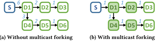
Figure 2: Example of how multicast flit forking reduces network traffic. The number on each link indicates the load of the link. Shaded routers fork the multicast flit.
